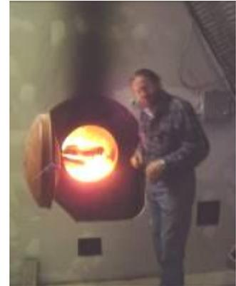
David Old checks the fire in the Garn Biomass burner for his recently constructed wood-drying kiln.
